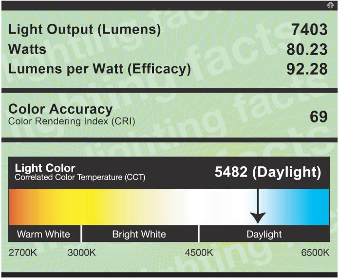
All results are according to IESNA LM-79-2008: *Approved Method for the Electrical and Photometric Testing of Solid-State Lighting.* The U.S. Department of Energy (DOE) verifies product test data and results.
