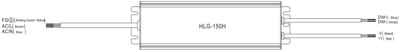
※ Built-in 3 in 1 dimming function, output constant current level can be adjusted through output cable by 1 ~ 10Vdc, 10V PWM signal or resistance between DIM+ and DIM-.
